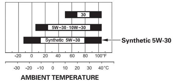
SAE 10W-30 or 5W-30 is recommended for general use. Use a full synthetic 5W-30 for starting/operating temperatures between 5°F (-15°C) and -13°F (-25°C). Other viscosities shown in the chart may be used when the average temperature in your area is within the indicated range.
