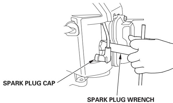
3. Inspect the spark plugs. Replace them if damaged, badly fouled, if the sealing washer is in poor condition, or if the electrode is worn.
