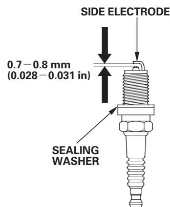
5. Install the spark plugs carefully, by hand, to avoid cross-threading.
