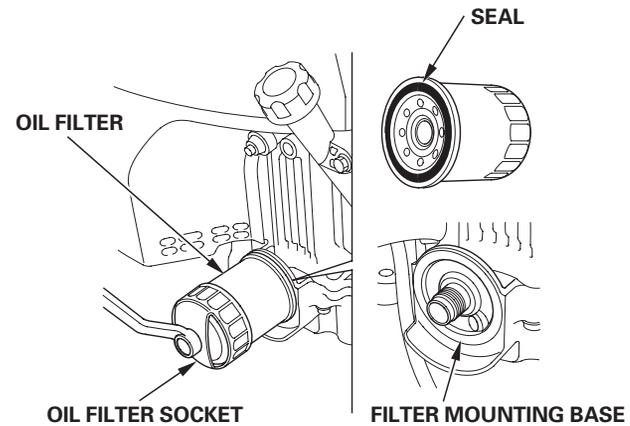
3. Clean the filter mounting base, and coat the seal of the new oil filter with clean engine oil.
